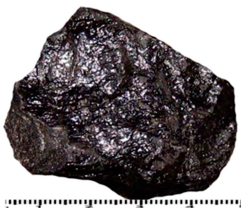
Phot. 8. Hydrocarbon coatings with sulphides on the slickenside
