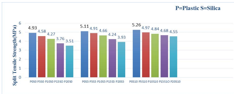
Fig. 5. Comparison of the split tensile strength of concrete mixtures prepared with varying percentages of e-plastic fine aggregate
