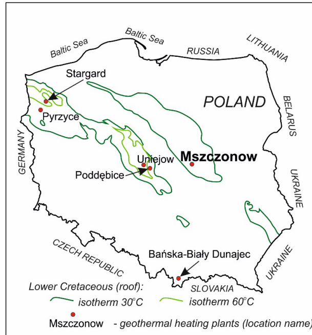
Fig. 1. Location of Polish geothermal heating plants. The Mszczonów, Uniejów and Poddębice exploit waters from the Lower Cretaceous, Pyrzyce and Stargard – from the Lower Jurassic, in Bańska-Biały Dunajec – from mainly Triassic sediments
