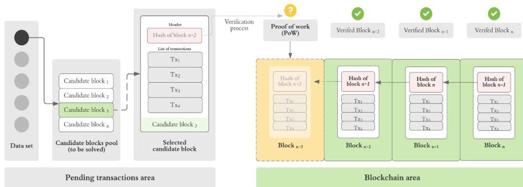
Fig. 2. Simplified scheme for adding new transactions to an existing blockchain with proof of work
