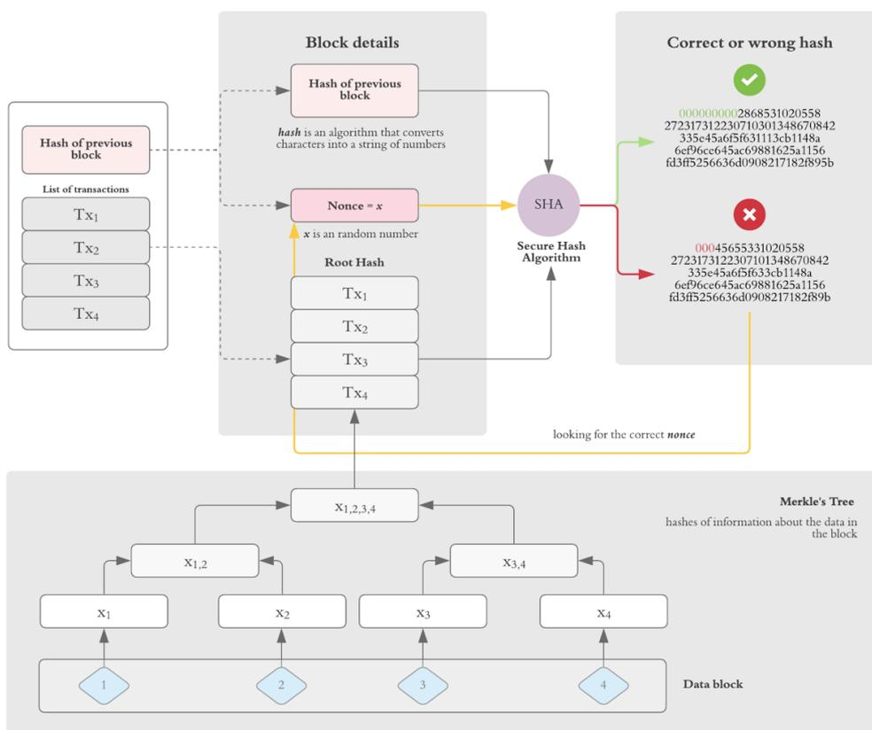
Fig. 3. A simplified diagram for adding a header to a pending block by solving a proof of work considering the Merkle tree problem
