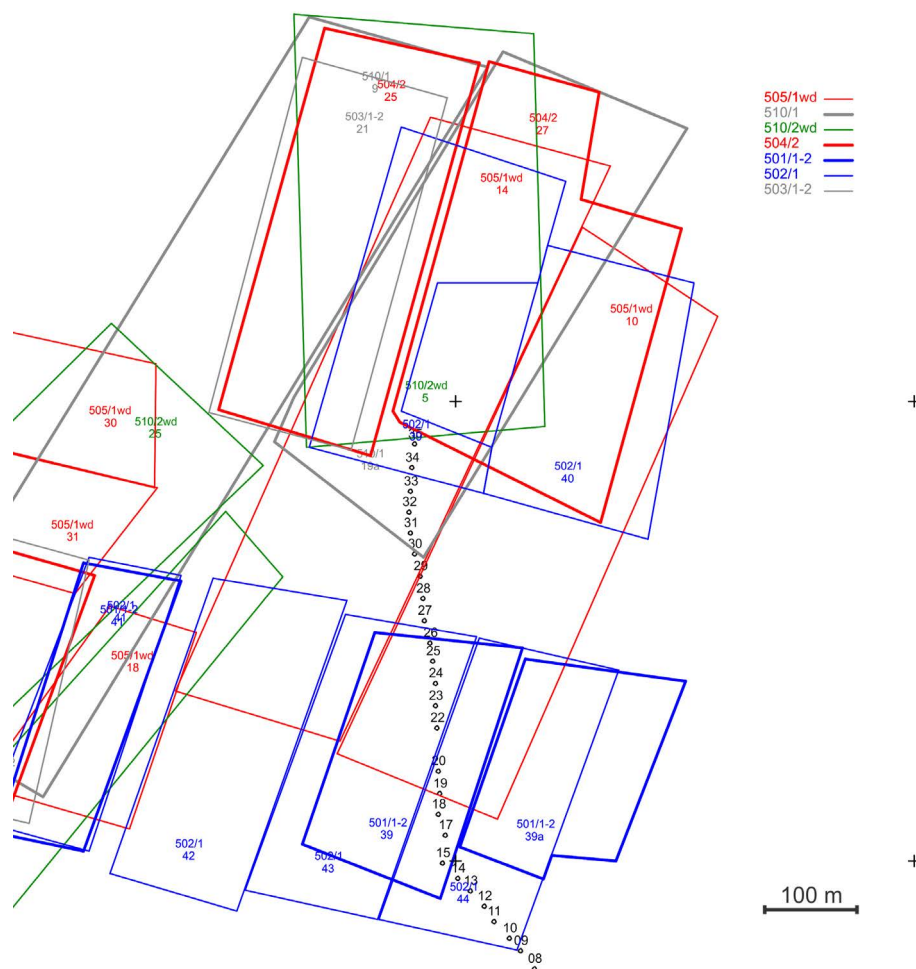
Fig. 9. The exploitation sites in the analyzed area of HCM 3 in the period Nov. 1985–Sept. 2005, with the positioning of the observation line
