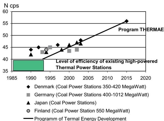
Fig. 2. Increase of efficiency of Coal Power Station
