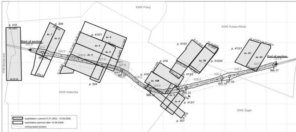
Fig. 3.1. Layout of coal exploitation performed in years 2003–2005 at area of A4 highway
