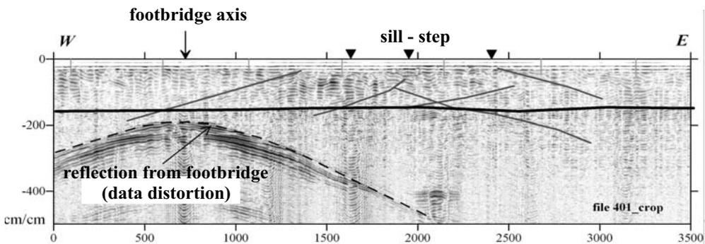
Fig. 6.4. Substrate discontinuities in the southern shoulder of A4 roadway (direction Katowice) at area of sill in GPR image (depth section)
