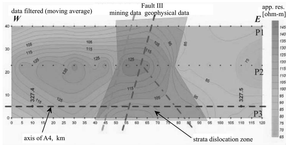
Fig. 5.2. Iso-ohm contours registered in bedrock during 1st series of resistivity measurements at segment from km 327.390 to km 327.510 (P1,P2,P3 – measurement profiles)
