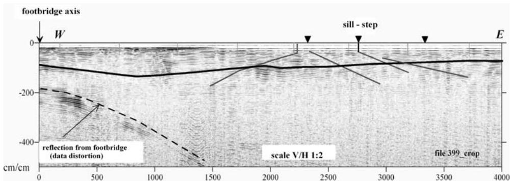
Fig. 6.3. Substrate discontinuities in the northern shoulder of A4 roadway (direction Wrocław) at area of sill in GPR image (depth section)
