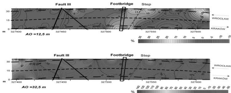
Fig. 6.2. Maps of soil and rock apparent resistivity changes (expressed as a percentage of initial values) between III and II measurement series (upper image – subsurface soil, bottom image – bedrock)
