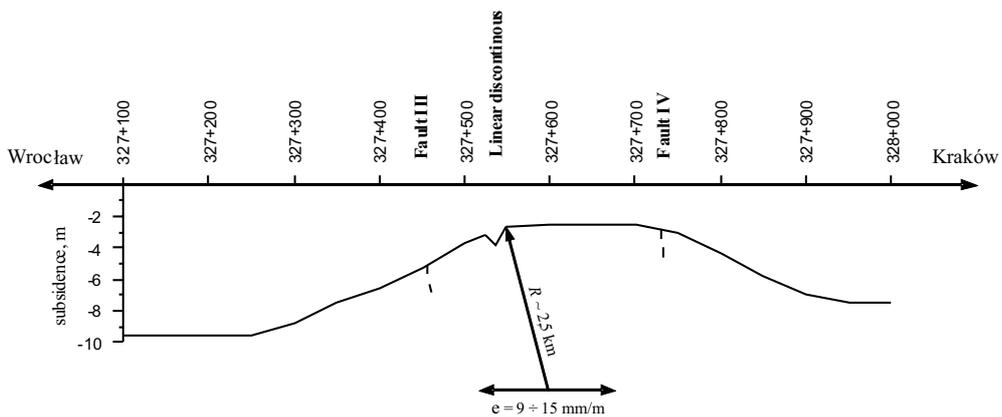
Fig. 4.1. Subsidence of surface in highway A4 axis before commencement of construction works at area of faults III and IV, due to performed exploitation and estimated horizontal deformation  $\epsilon$
