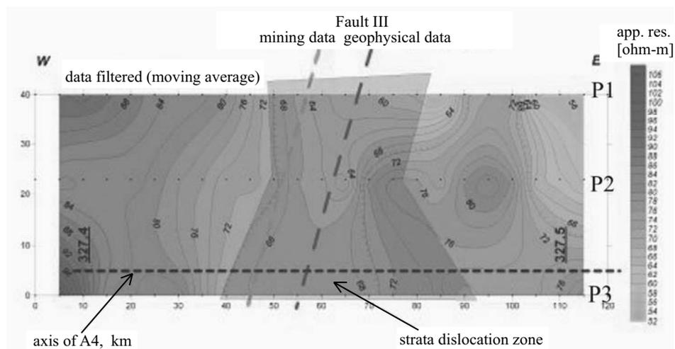
Fig. 5.1. Iso-ohm contours registered in subsurface soil during I<sup>st</sup> series of resistivity measurements at segment in km 327.390–327.510 (P1, P2,P3 – measurement profiles)
