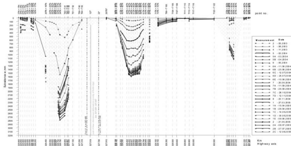
Fig. 4.2. Measured subsidence along the longitudinal axis of A4 highway in period from 03.2003 to 12.08.2005
