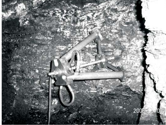
Fig. 8. The Expanding bolt system for in-situ test on C1 coal seam
