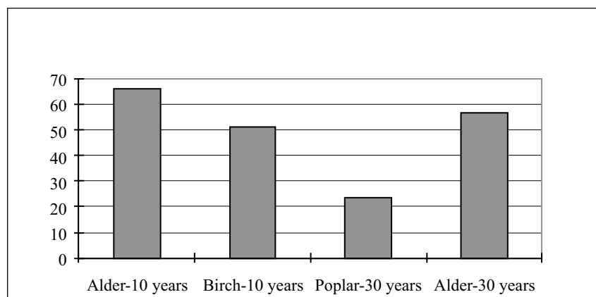
Fig. 2. Accumulation of total nitrogen (net value) in horizons Olfh and A of soils in experimental fields on the external part of the waste heap of the Lignite Mine "Turów" [kg/ha/year]
