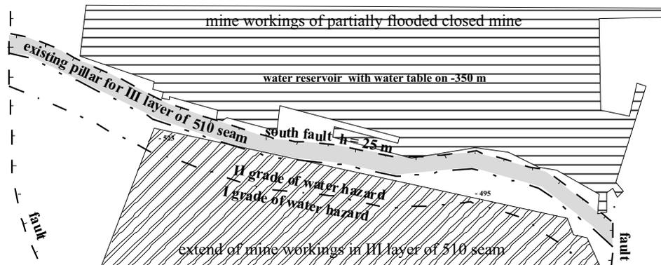
Fig. 2.2. Situation sketch in the area of water reservoir formed in the abandoned mine with safety pillar separating mine workings within the layer III of the seam 510 from the zone of south fault before water table rebound in the reservoir to the ordinate of  $-200$  m
