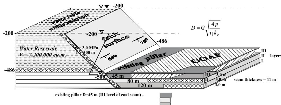
Fig. 2.3. The scheme for the exploitation designed within the fault wall throw in the vicinity of water reservoir of very large capacity and calculations for critical pillar dimension
