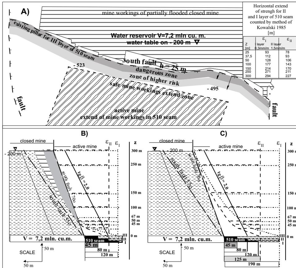
Fig. 3.1. The scheme of safety spheres indication on the maps A), the reach of rock mass deformation while preserving distances of designed exploitation from the source of water hazard according to calculated critical dimension of the safety pillar B), and after graphically position correct of the exploitation front away from a reservoir C)
