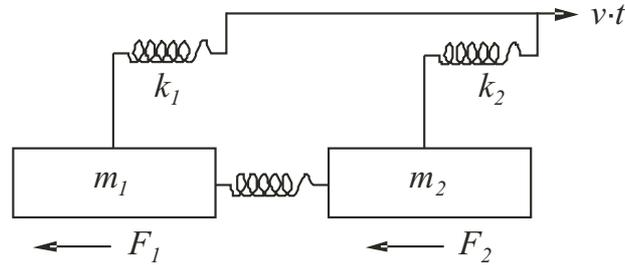
Fig. 1. Model of moving masses on the friction surface
