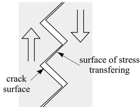
Fig. 3. The surface of crack and the surface by which the stresses be transferred
