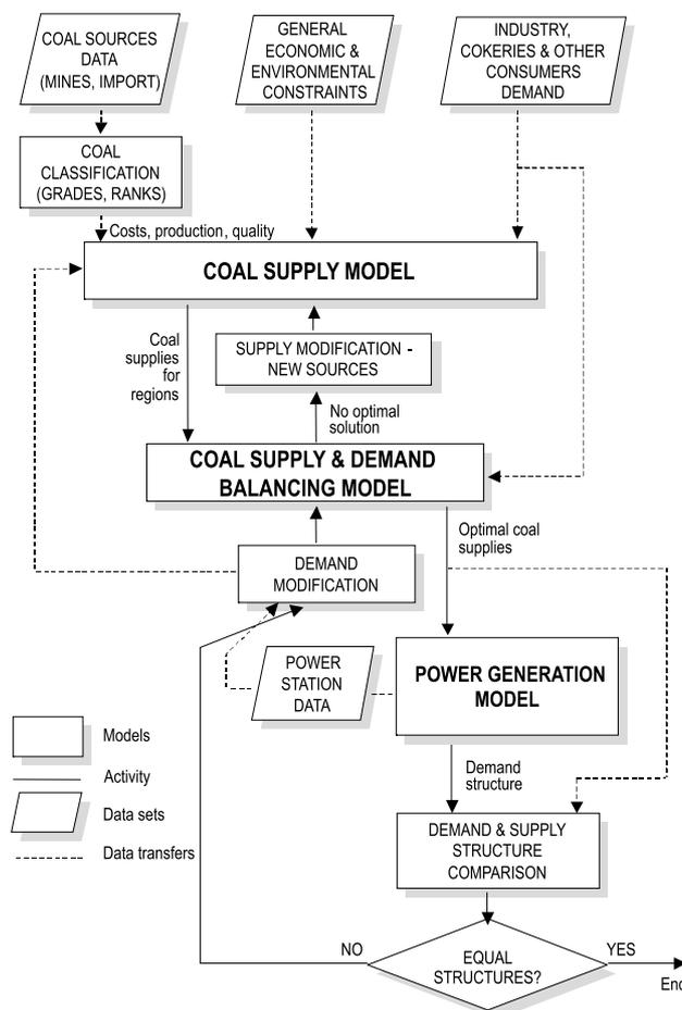
Fig. 5. General framework of models co-operation within coal balancing system for the country level
