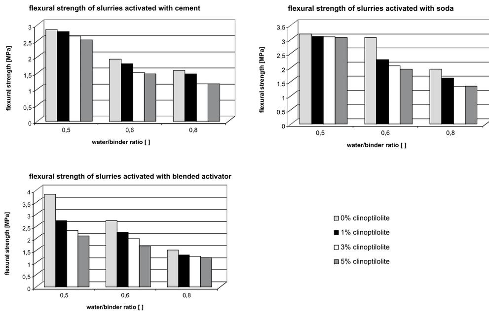
Fig. 10. Flexural strength of hardened slurries after 7 days of curing in water
