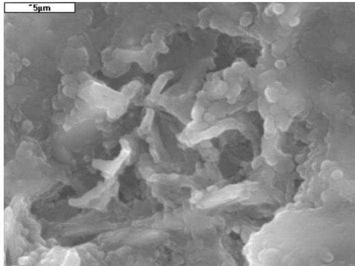
Fig. 14. Elongated features within cement activated, 5% clinoptilolite paste;
