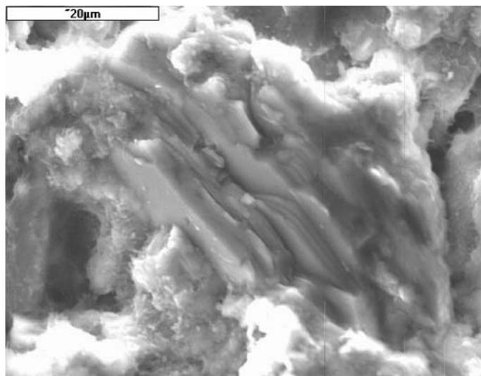
Fig. 16. Portlandite and fibrous C-S-H visible in cement activated 1% clinoptilolite slag paste; cured in water for 28 days
