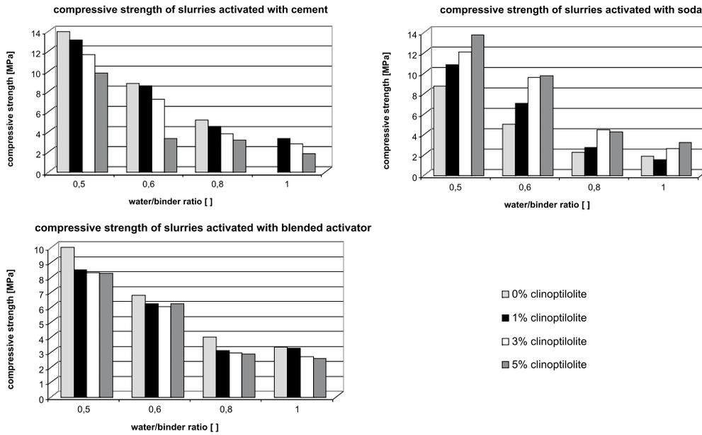
Fig. 9. Compressive strength of hardened slurries after 7 days of curing in water
