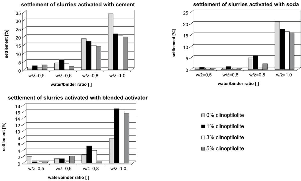
Fig. 2. Settlement of slurries modified with clinoptilolite
