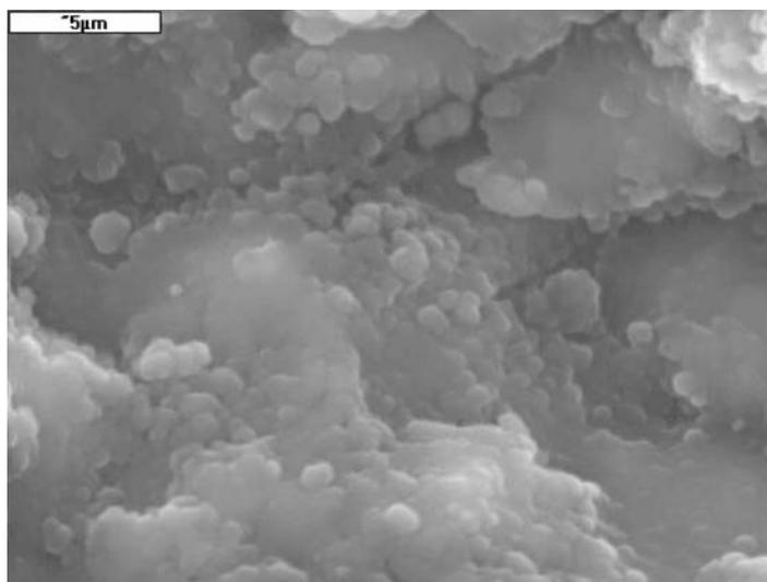
Fig. 11. C-S-H phase in paste activated with soda modified with 1% clinoptilolite addition; cured 120 days in water
