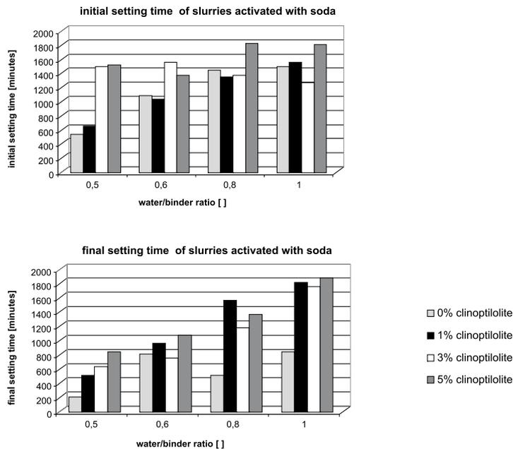
Fig. 6. Initial and final setting time for slurries activated with soda
