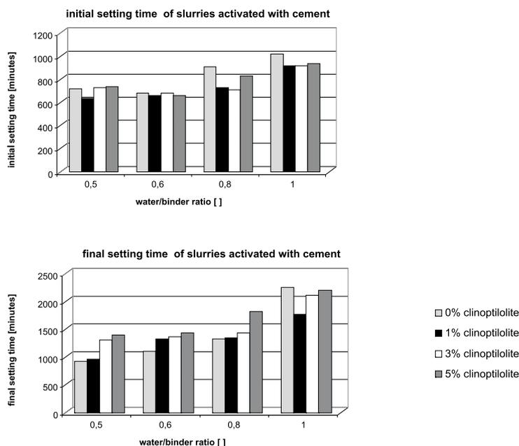
Fig 4. Initial and final setting time for slurries activated with 10% of cement
