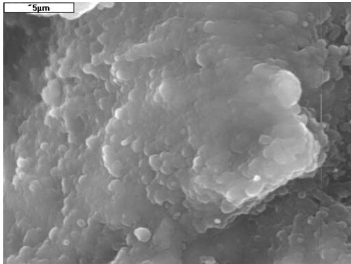
Fig. 12. C-S-H phase in paste activated with cement, modified with 1% clinoptilolite addition; cured 120 days in water
