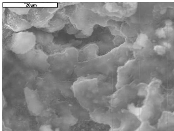
Fig. 15. Soda activated slag paste modified with 1% addition of clinoptilolite – C-S-H of C/S ratio 0.9;
