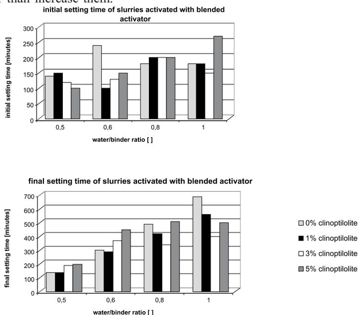
Fig. 8. Inital and final setting times for slurries activated with blended activator
