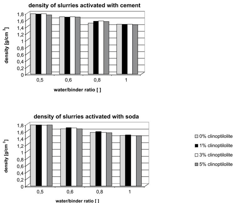
Fig. 1. Density of slurries modified with clinoptilolite
