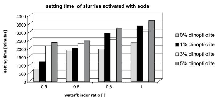
Fig. 7. Setting time for slurries activated with soda
