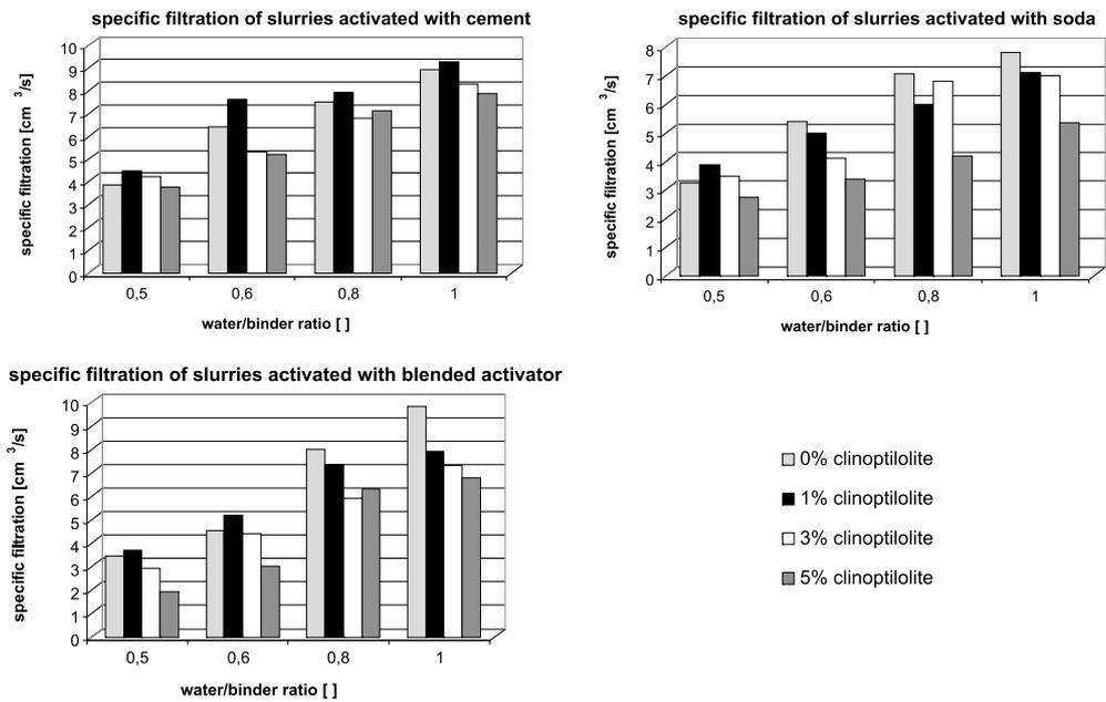
Fig. 3. Filtration of slurries modified with clinoptilolite
