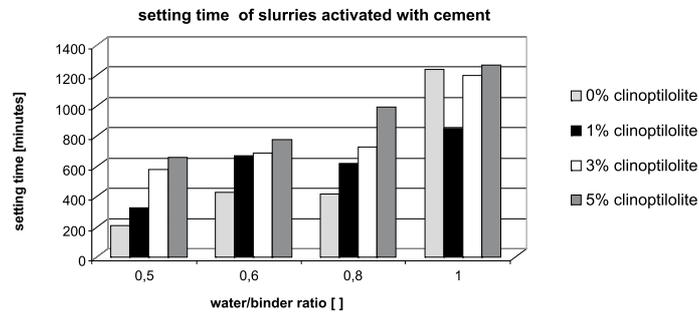
Fig. 5. Setting time of slurries activated with cement
