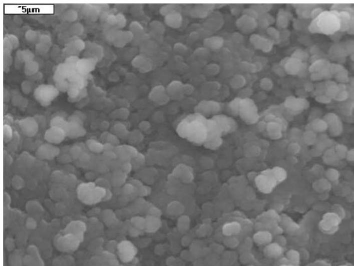
Fig. 13. C-S-H phase in paste activated with blended activator modified with 5% clinoptilolite addition; cured in water for 120 days
