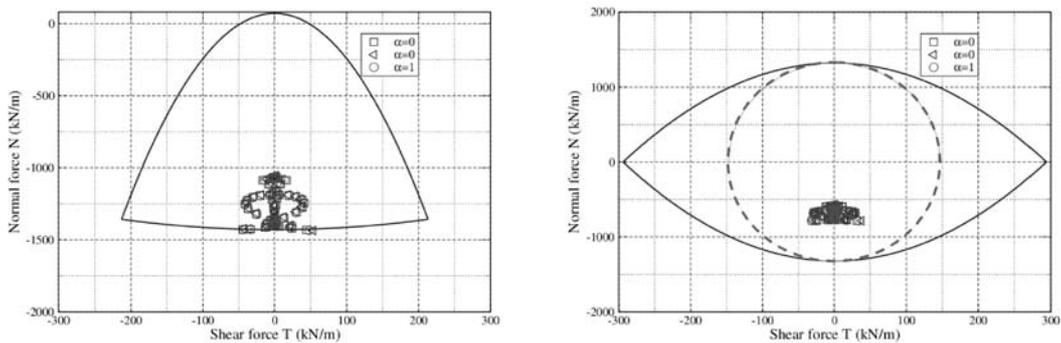
Fig. 11. Shear force vs. normal force for shotcrete (left) and steel ribs (right) (case 2).
