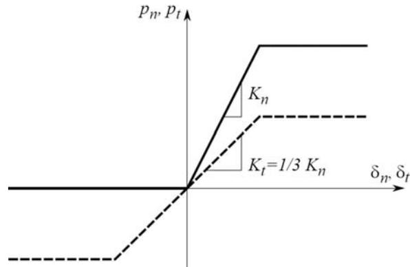
Fig. 2. Constitutive relationship of the springs representing the ground reaction in the bedded-spring model  $p_n$  and  $p_t$  represent the normal and tangential load,  $\delta_n$  and  $\delta_t$  the normal and tangential displacement and  $K_n$  and  $K_t$  the normal and tangential stiffness
