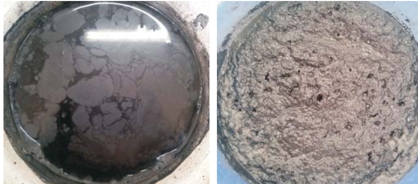
Fig. 4. Foam images using air bubbles (on the left) and oily bubbles (on the right)
