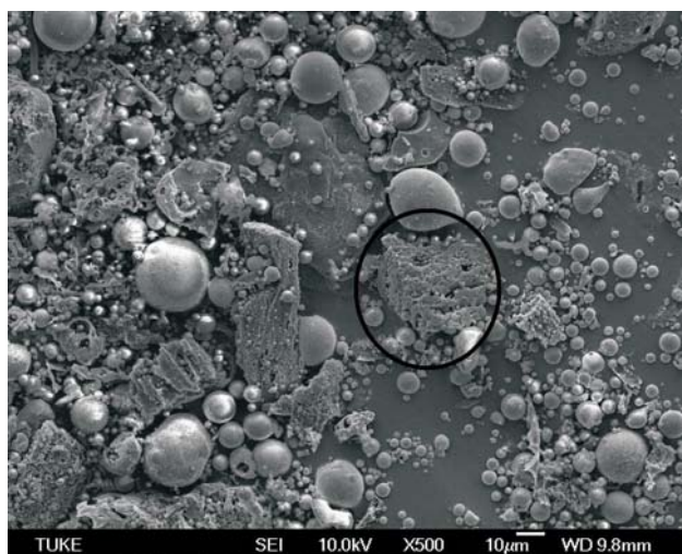
Fig. 1. Morphology of deposit fly ash (SEM)
