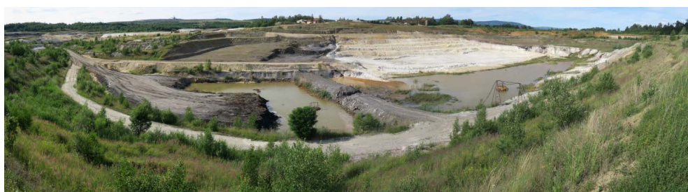
Fig. 2. Kaolin deposit Božičany-Osmosa in the Karlovy Vary region, producing all grades of kaolin (kaolin for production of porcelain and fine ceramics, for other ceramics manufacturing, and titanium-bearing). Elevation of medium-grained muscovite-biotite granite weathered in Tertiary, since Late Oligocene lignite seam is in direct kaolin overburden Phot. Jaromír Starý 2016
