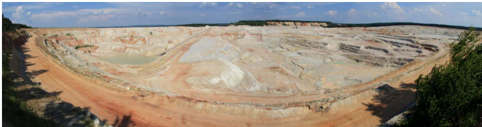
Fig. 4. Kaolin open pit mine Kaznějov in the Plzeň region extracting two deposits: Kaznějov-South and Lomnička-Kaznějov. It is largest open pit kaolin mine in the Czech Republic, producing mostly paper-grade kaolin and kaolin for other ceramics. Parent rock is Late Carboniferous arkose Phot. Jaromír Starý 2016
