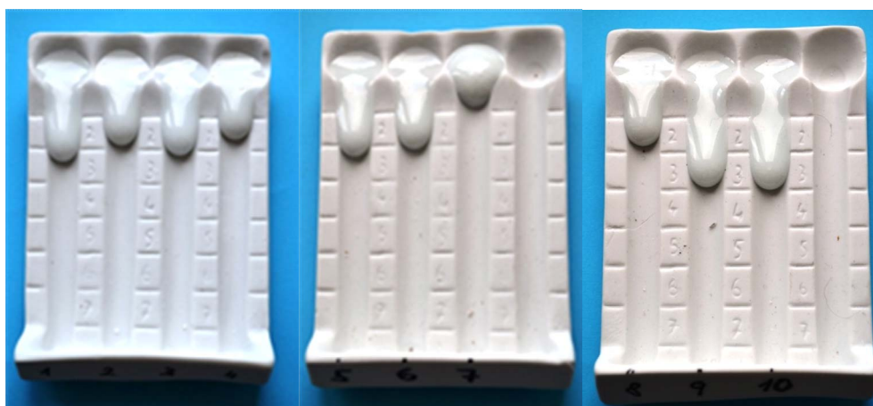
Fig. 14. Flowability of glass prepared in accordance with 10 formulas
